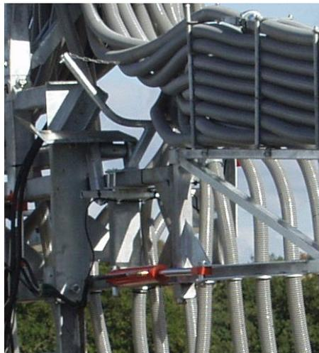
The spreader hose boom is of very robust design and is fitted with trapezoidal suspension which effectively compensates for the unevenness and shocks that can easily damage rigidly mounted booms. The trapezoidal suspension thus increases the operating life of the boom.
